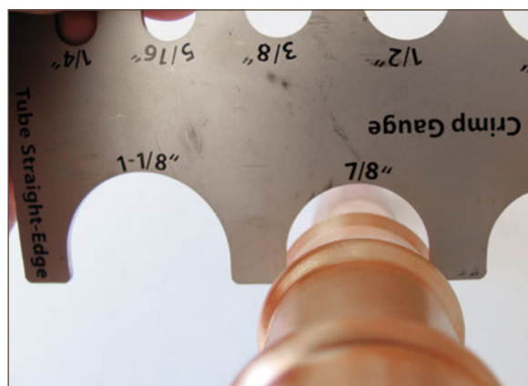
Figure 11.22. Un-crimped or improperly crimped fitting
