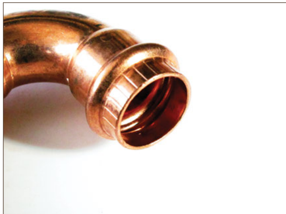
Figure 11.11. Press fitting (NOTE: Missing o-ring)
